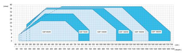
Fig. 1 X = Caudal Y = Presion en camara de combustion (mbar)
